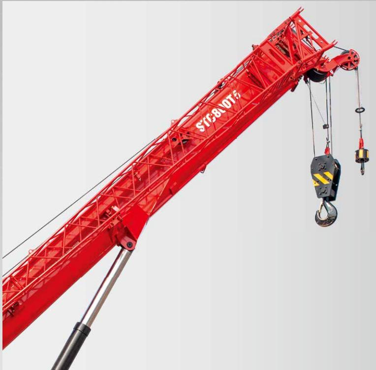
Five section large cross section boom, full extension length 49.5m at 42m radius, 17.5m bi-fold jib available. The lifting performance leads in industry.
