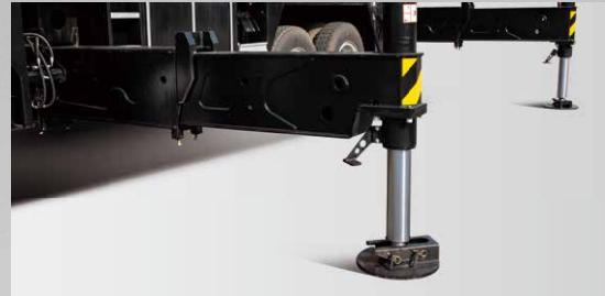
Outriggers extend to 8m in full span, making lifting operation more stable. Newly developed half extension mechanism makes the crane more adaptable to work at constricted area.
