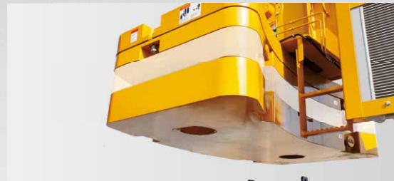
Fixed CW 3t, movable CW 12t. The crane can travel with 15t CW on board at low speed (<20km/h) in short distance.
