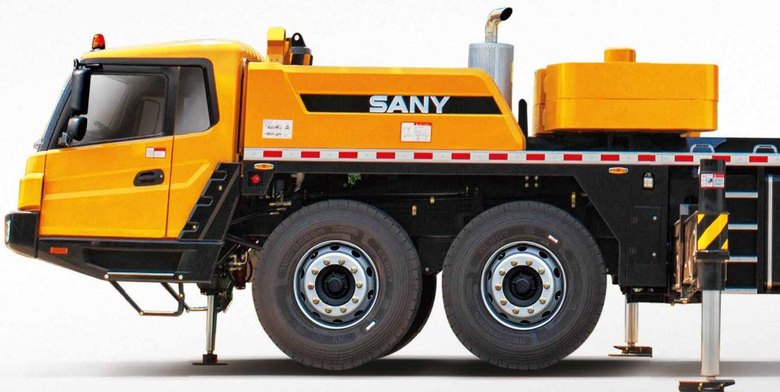
G Class, ground clearance 340mm, approach / departure angle 19/15°, all axle steering, outstanding travel flexibility.
