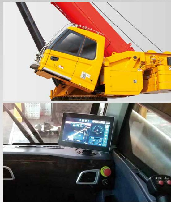
0~20° tilttable cab, relieving fatigue in long time operation.
